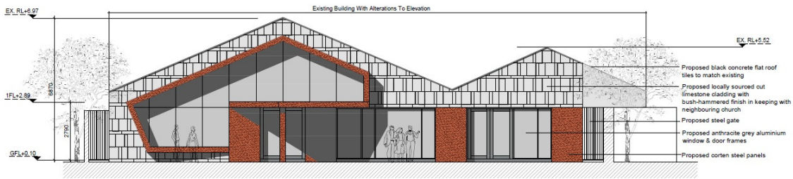
Fig5. Proposed Library. Front Elevation
