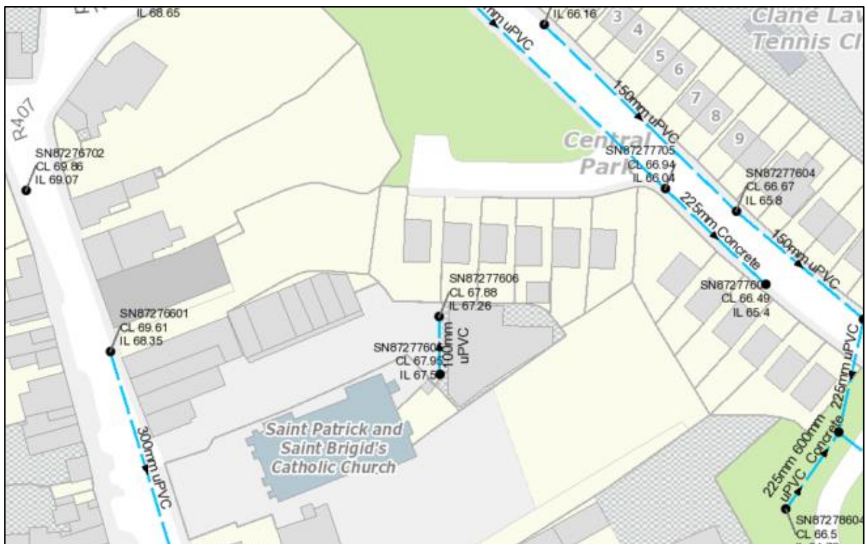
Figure 3 | Existing Surface Water Drainage Network
